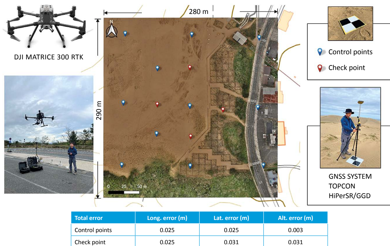
Fig. 2 Topographic data acquisition along a 280 m × 290 m square using the DJI MATRICE 300RTK UAV in combination with Ground Control Points and Check Points recorded by GNSS commercialized by TOPCON.
