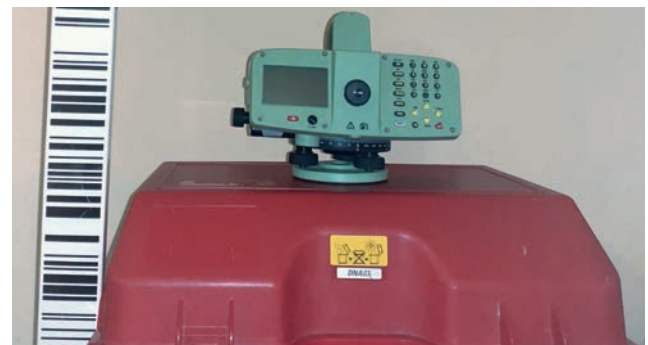
Fig. 3 The equipment, Leica DNA03™ and the staff (Professional 3000 series), that was used for the leveling measurements.
